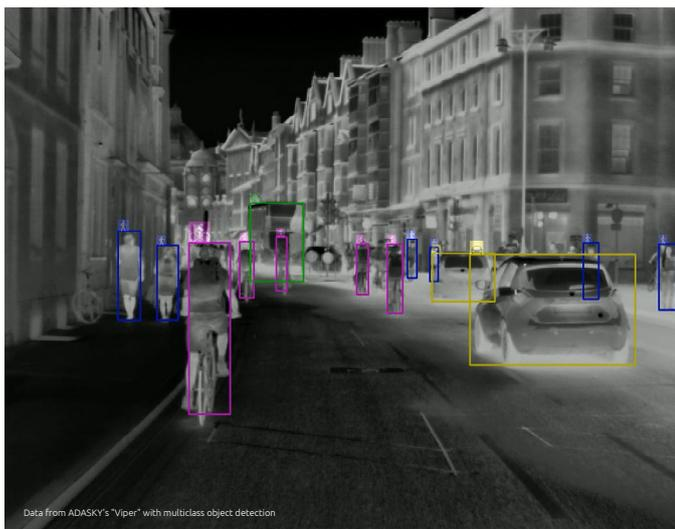
every object, living or inanimate. Each object emits a unique thermal signature that allows for differentiation to a very high degree of accuracy ( $\pm 0.05^{\circ}\text{C}$ ), and with Viper, a high resolution, grayscale 14-bit video image can be achieved. Incredibly, thermal imaging cameras are the only technology that can sense and classify living beings (pedestrians, bicyclists and animals) far enough in advance to allow for the automated vehicle or human driver to safely react at night.
