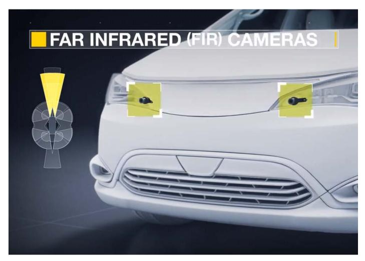
AdaSky and Magneti Marelli integrate FIR into a vehicle's headlights for the first time
