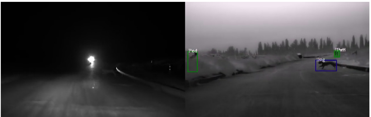
State-of-the-art camera with low light sensitivity (Featuring the sony IMX174 CMOS image sensor)
